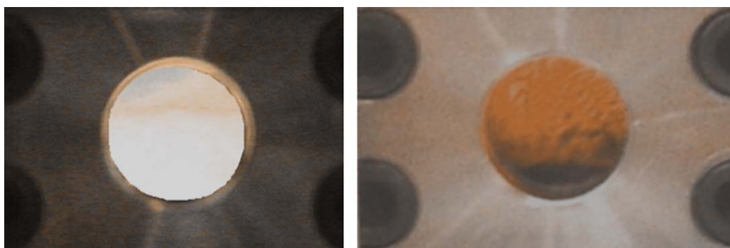
Fig. 2. (Left) the slurry containing cis -2-pentenitrile, surfactant, Pd and Ru precursor solution at 298 K in liquid \text{CO}_2 ; (right) most slurry disappeared with formation of a brown 'solution' containing noble metal(s) nanoparticles in supercritical \text{CO}_2 (~140 bar), 20 bar \text{H}_2 at 313 K.
